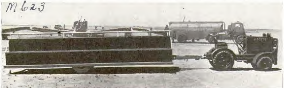
Trailer "bus," towed by tiny tractor, saves time of cadets when large groups are moved long distances
